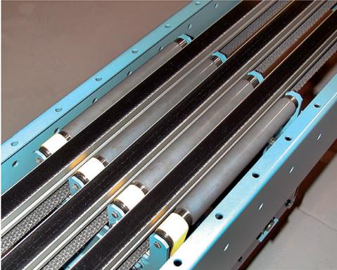
A series of narrow belts, each with its own take-up, span the length of the conveyor. High-friction rollers rise up between the belts, accurately diverting small product at right angles to one side or both sides.
