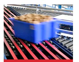
A series of narrow belts, each with its own take-up, span the length of the conveyor. High-friction divert wheels rise between the belts, accurately diverting product at a 30-degree angle. The NBS 30 is as efficient as it is fast—divert wheels are driven from the main conveyor, eliminating the need for extra drives.
