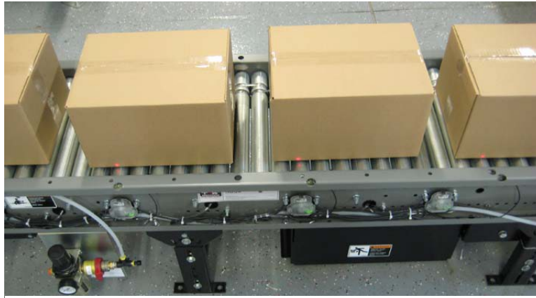
Non-contact zero pressure zones
