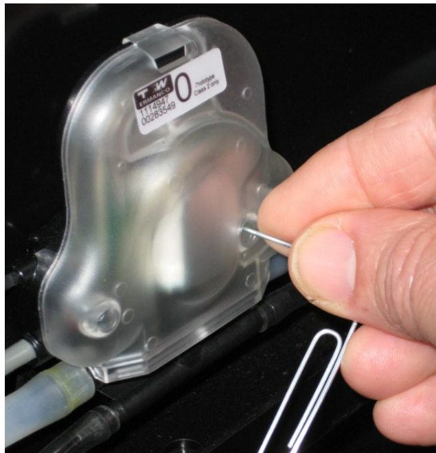
Switching logic modes with paper clip
