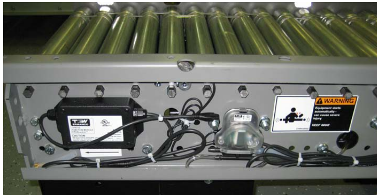
Release function module at discharge end of NBC V-Belt conveyor
