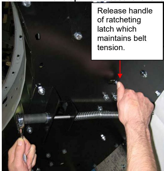
Generation 1 – Take-up with release lever shown
