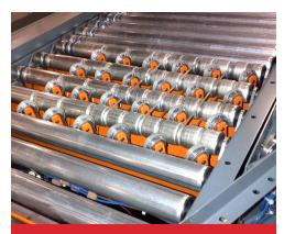
Adjustable speeds between 25 FPM to the maximum speed of 180 FPM.
