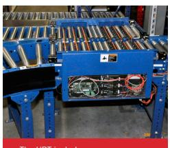
The UBT includes standard features such as low maintenance air bags and precision linear bearings that guide the transfer as it raises and lowers, ensuring that the transfer surface remains level to minimize product skewing.
