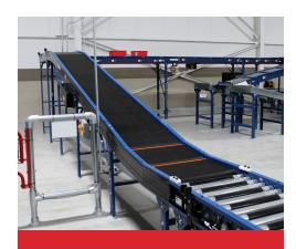
Belt conveyors provide smooth, continuous flow of product under positive control and are commonly used to change elevation by inclining or declining.
