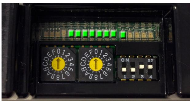
3. Power OFF the IB-E and set the rotary switches and the DIP switches to the previous (or other operational) settings.
