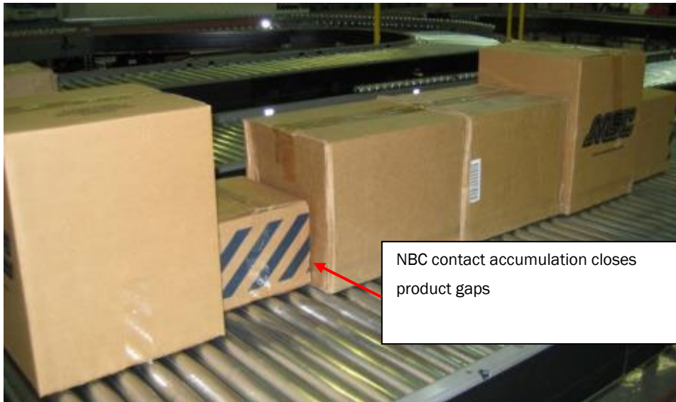
NBC flat belt contact accumulation
