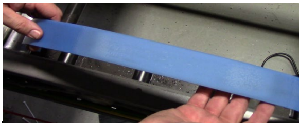
Top side of blue urethane belt after weld
