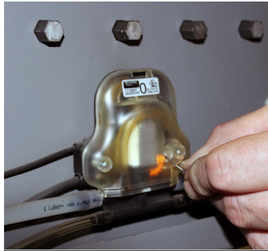
Amber light indicates progressive mode.
