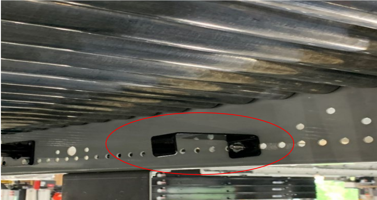
Skew bed skew guard storage location.
