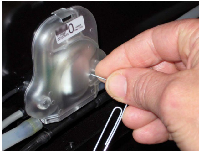
Switching logic modes with paper clip
