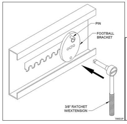
cams must be set vertical and aligned the same on both sides. See Caution and pictures below.
