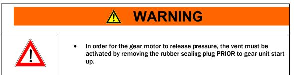
Please check you gear unit for a vent and if applicable to your product, remove the sealing plug to activate. "https://www5.nord.com" Operation Manual for Gear Units (B1000).
