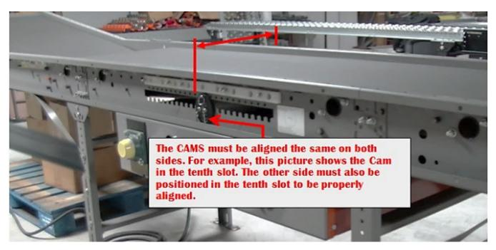
The Cams must be aligned the same on both sides.
