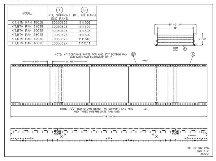
Bottom pans are safety covers that provide operator protection from running belts and debris, and are highly recommended up to 8' from the floor.
