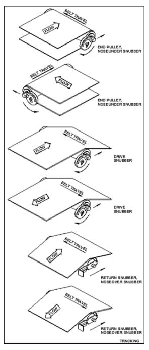
**NOTE:** Flow refers to belt surface flow direction not necessarily product flow.
