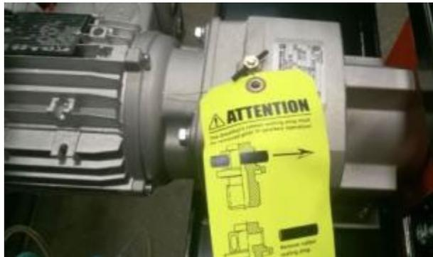
**Note:** Yellow tags may be tucked out of sight. Please inspect all motors for a vent and remove sealing plug, if present, to activate.
