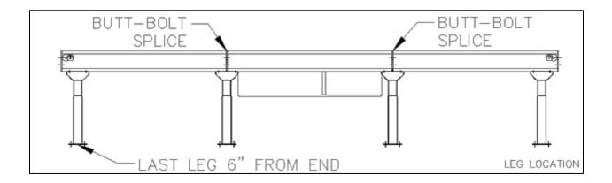
Leg elevations are shown on the elevation drawings. Leg elevation can also be set by subtracting 6-3/8" from the desired top of belt elevation.
