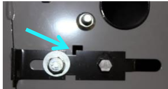
Slide snubber bracket over to align square holes. (Mid-point Location)
