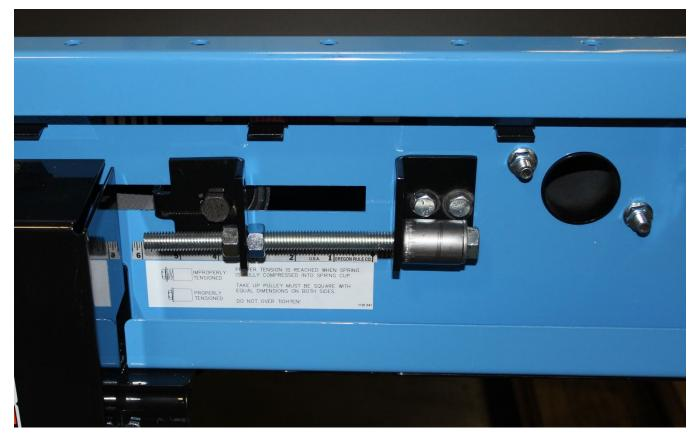
Proper tension has been reached when spring is fully compressed into spring cup.
