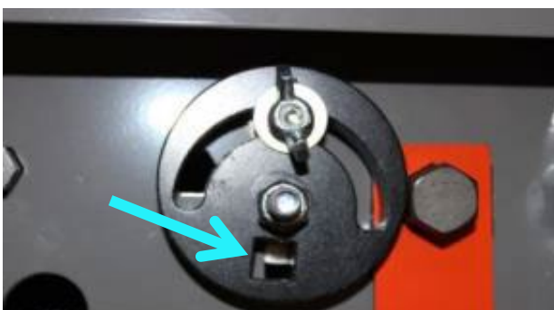
Move CAM over to align square holes. (Mid-point Location)
