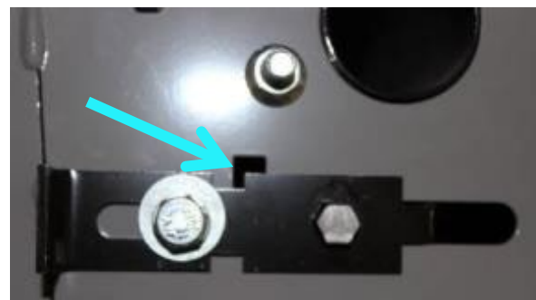
Slide snubber bracket over to align square holes. (Mid-point Location)
