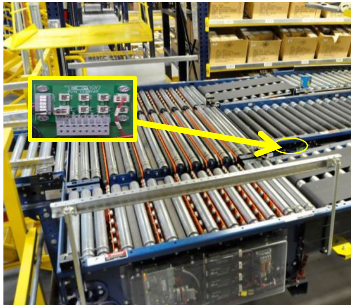
PCB Connector General Location on Induction Bed.
