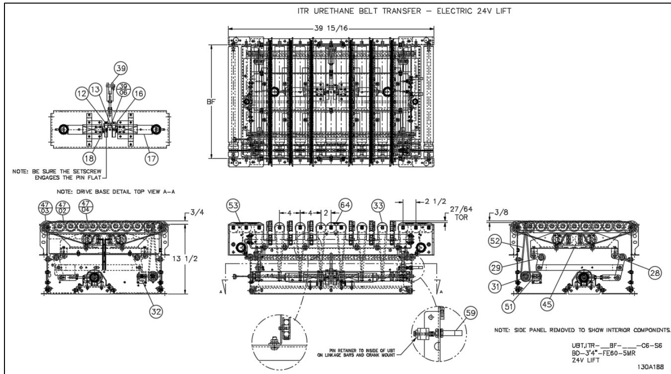
***17.48.1 Replacement Parts - ITR UBT (Electric Lift) - Mechanical Components 5s & 6s***
