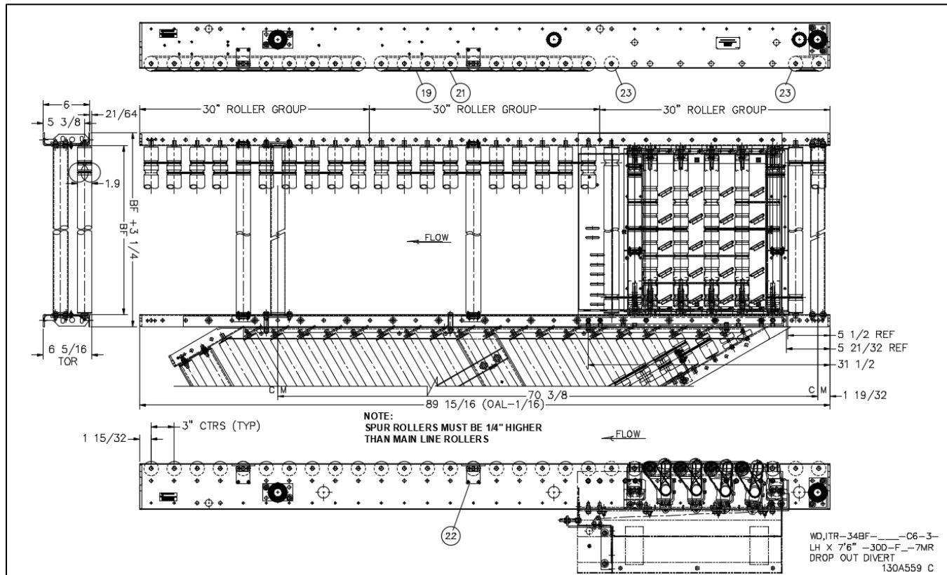
*a) Replacement Parts - ITR Wheel Divert, CBM-105, 3RC (Pneumatic)*
