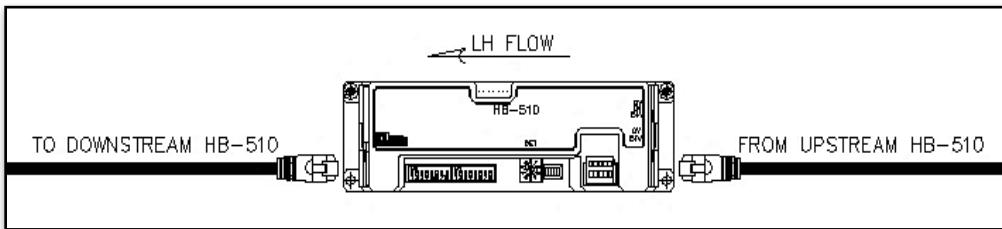
Figure 4 – HB-510 Communication Cable RH Flow
