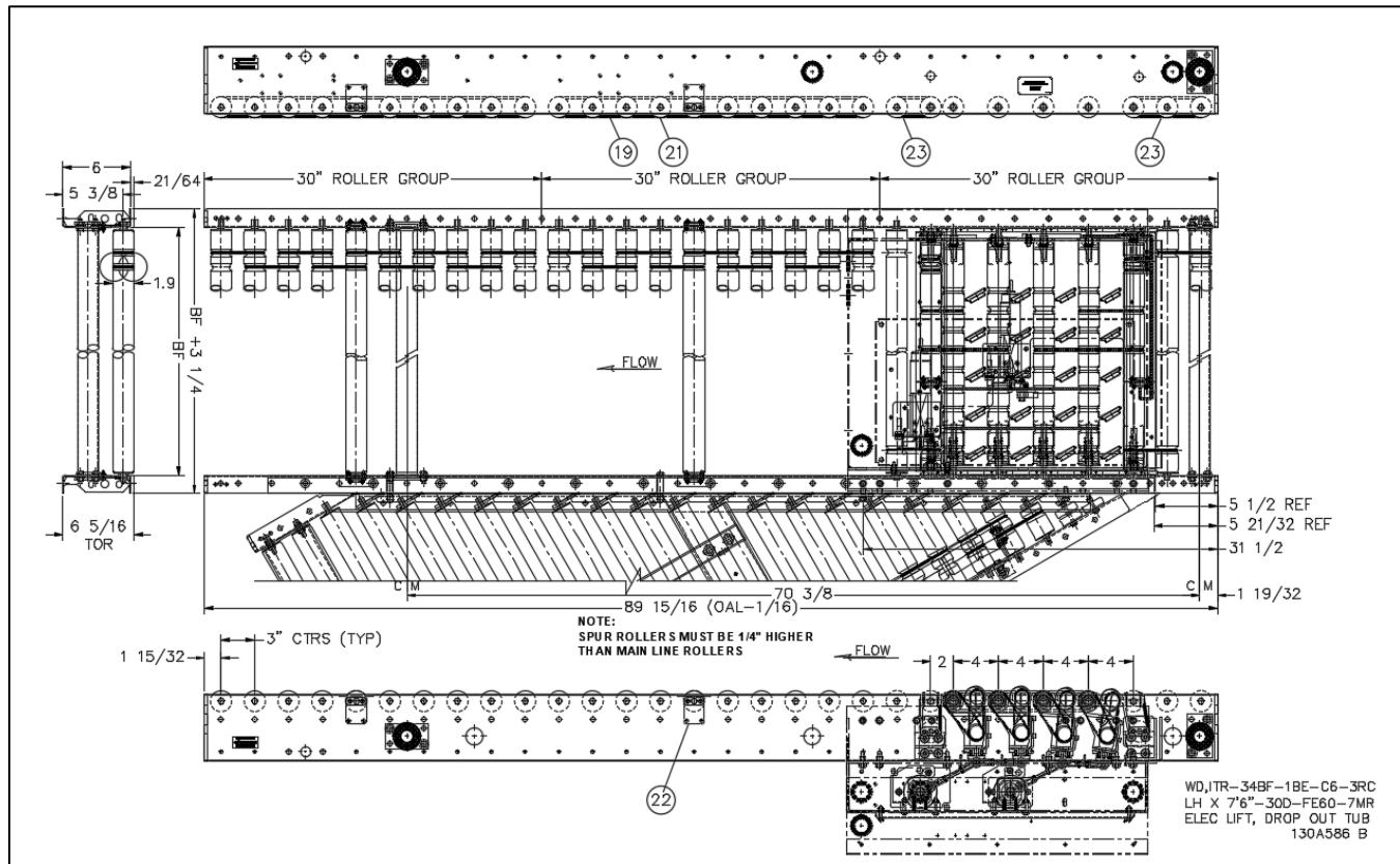
**17.42.1 Replacement Parts - ITR Wheel Divert, IB-E03, 3RC (Electric Lift)**
