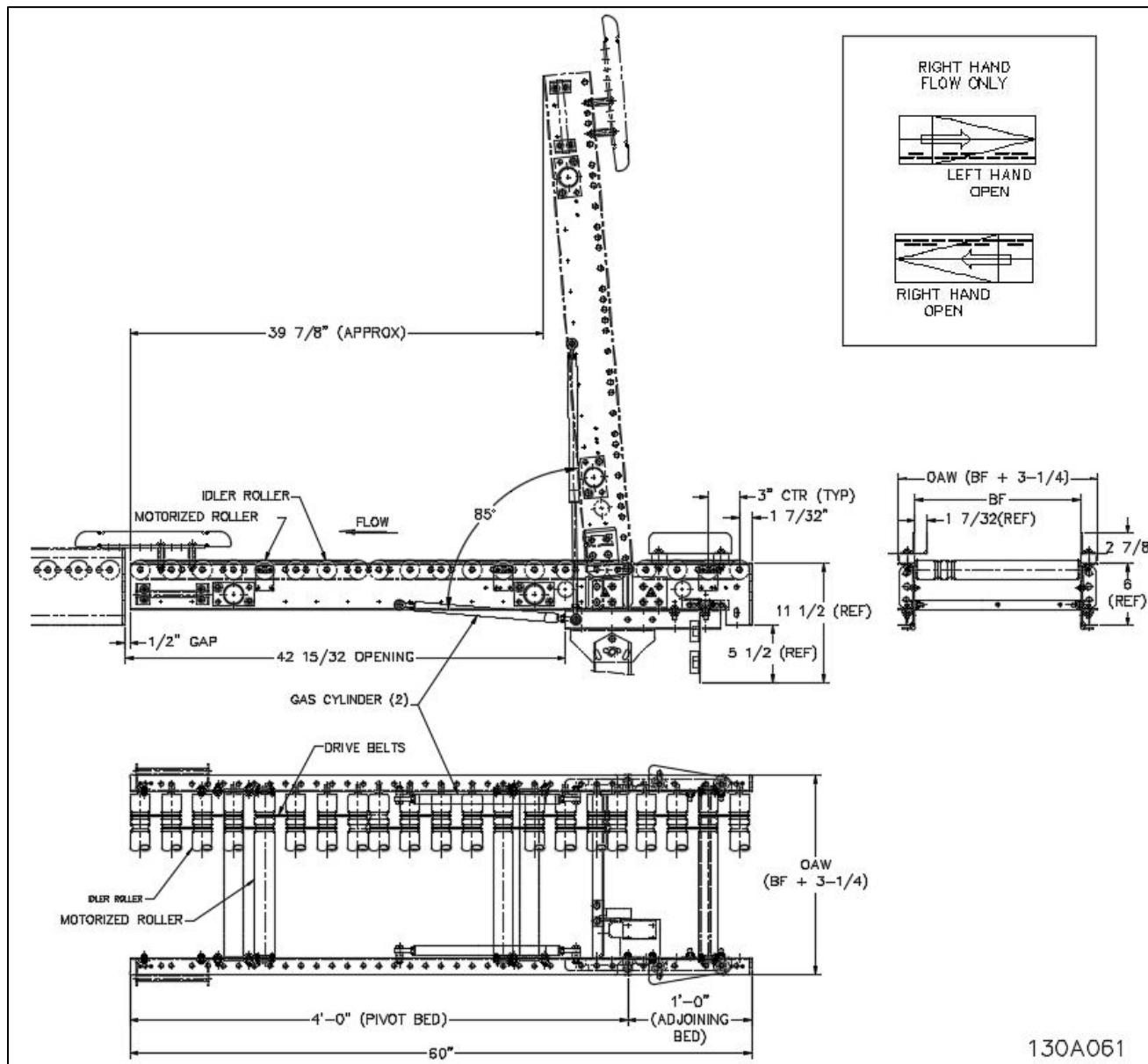
The gate provides a break in the conveyor line for pedestrian traffic. The power source must be from the charge side. The gate consists of a 4' pivoting bed and a 1' adjoining bed. Gates are available in right hand and left-hand lifts.
