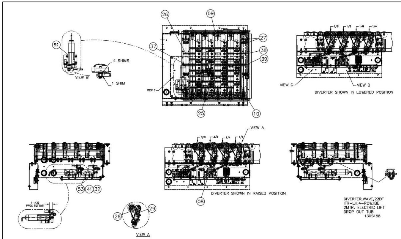
***17.43.1 Replacement Parts - ITR Wheel Diverter (Electric Lift) Components***
