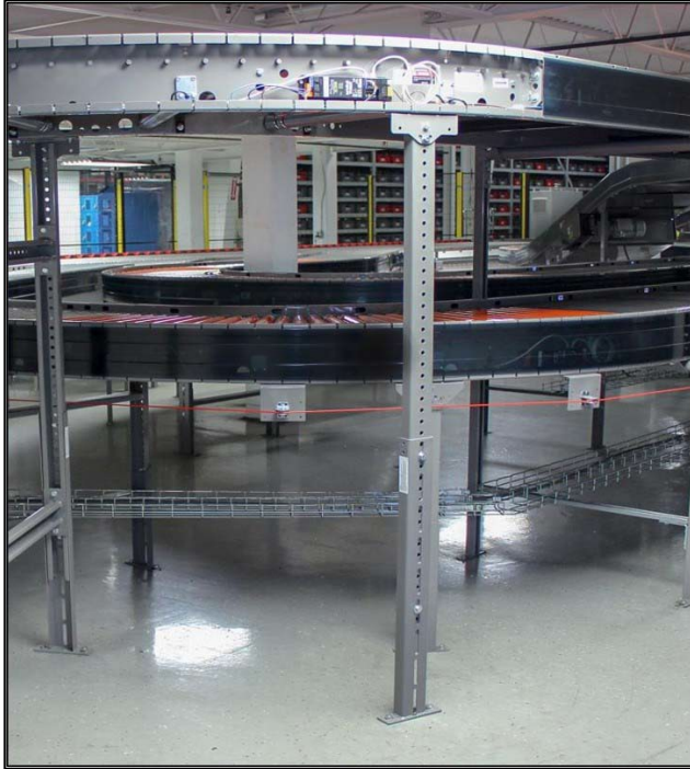
Single leg RF support on 90° ITR curve.
