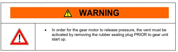
Please check you gear unit for a vent and if applicable to your product, remove the sealing plug to activate. "https://www5.nord.com" Operation Manual for Gear Units (B1000).
