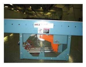
All belts must pass over any return rollers positioned to minimize belt sag and through holes in crossmembers.
