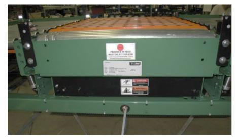
An identification label is attached to the charged end of the center Bed of each ITR Pick Zone Module.
