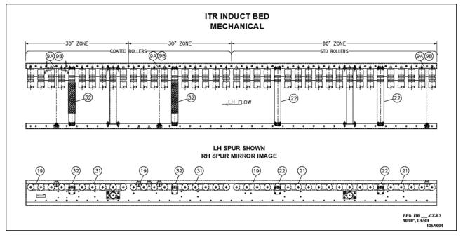
The IntelliROL Pick Zone Module starts with the Induction Bed. The Induct Bed gaps the product so it can be transferred.
