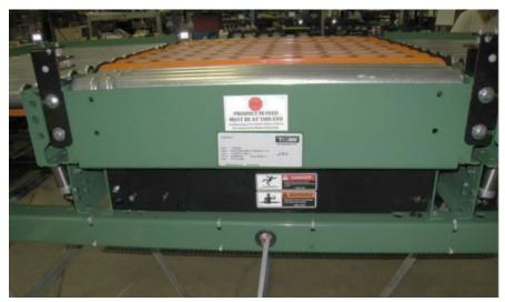
An identification label is attached to the charged end of the center Bed of each ITR Pick Zone Module.
