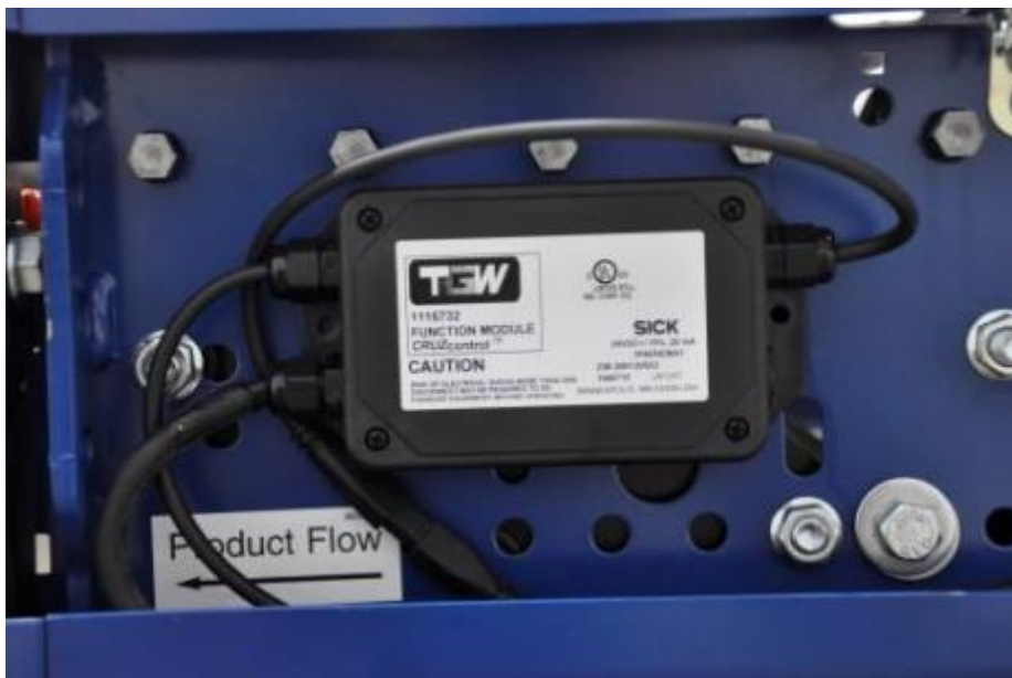
Release function module at discharge end of NBC conveyor part number 1116732
