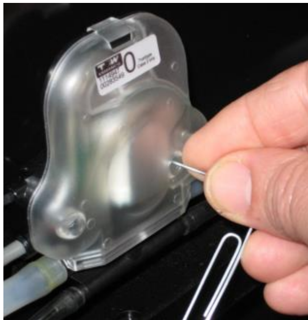
Switching logic modes with paper clip
