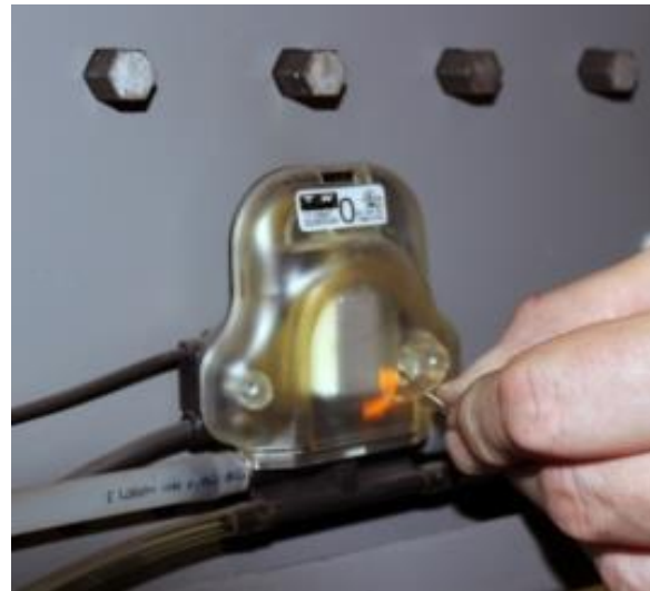
Amber light indicates progressive mode.
