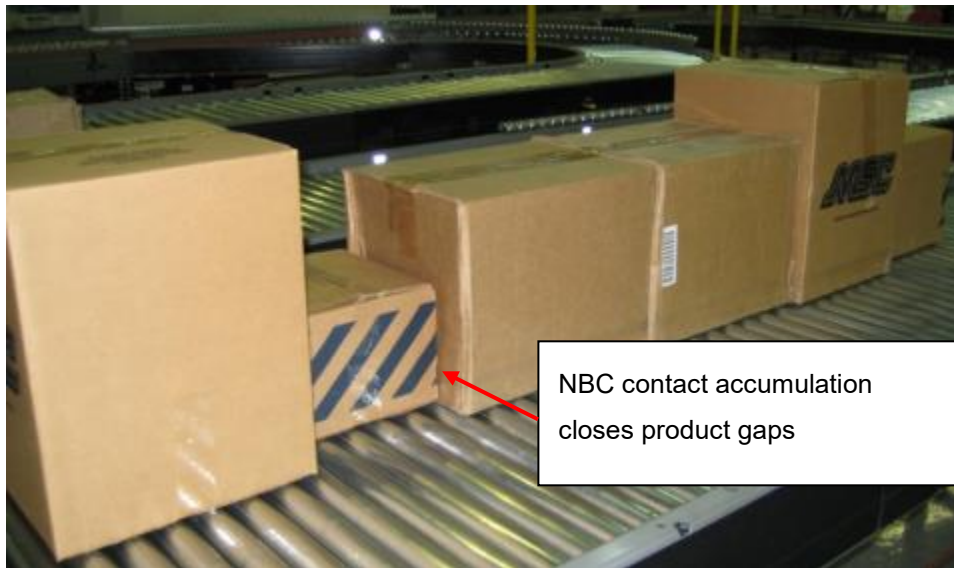
NBC flat belt contact accumulation
