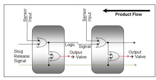
Figure 23: Progressive Accumulation Logic
