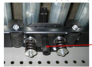
Rotate back to low side of Cam
