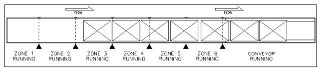
There is no gap between released products; assuming conveyor speeds (accumulation conveyor and downstream conveyor) are identical. The Progressive Logic discharge functions the same as a Slug Release. Initiating the Slug Release will also result in all products releasing, regardless of zone conditions. In the progressive release mode for contact accumulation, it is extremely important to set every 5th logic module to basic.
