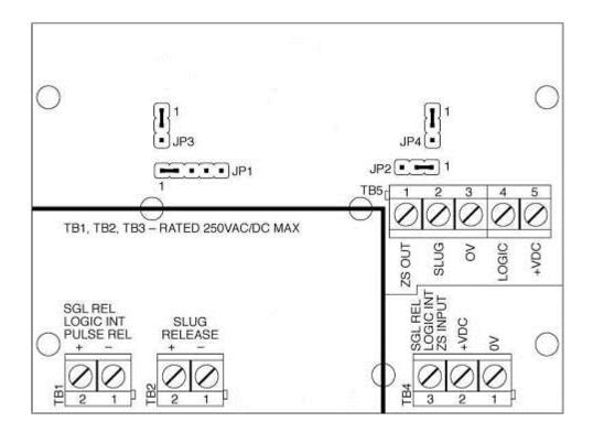
Figure 7: Release Function Module Circuit
