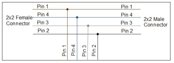
Figure 26: Power Interrupt Wiring
