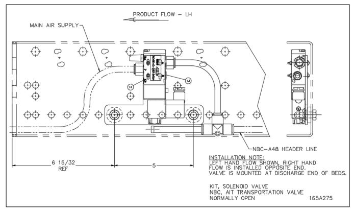
The Solenoid Valve Kit is controlled by an external signal from the primary control system supplied by the purchaser. The Solenoid Valve Kit is typically mounted near the last NBC contact accumulation
