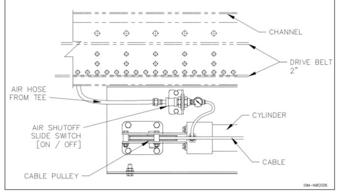
500 lb.-AT Air Sleeve Valve Assembly
