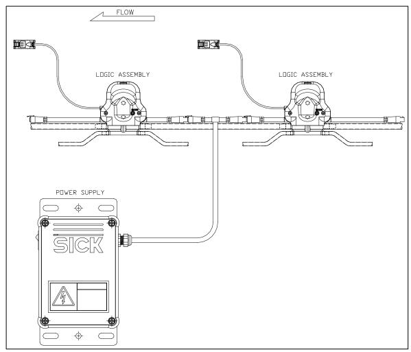
Figure 8: Two Logic Assemblies using a T Cable
