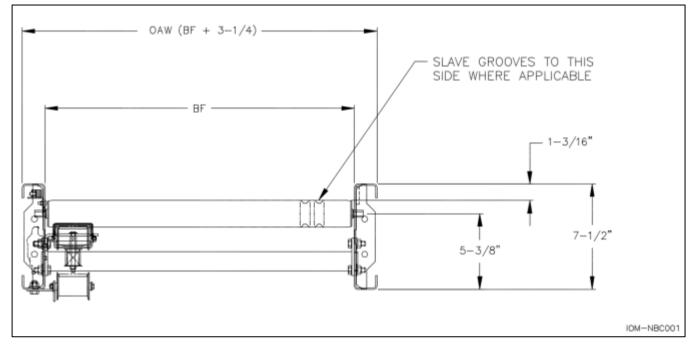
NBC accumulation with CRUZchannel rollers low
