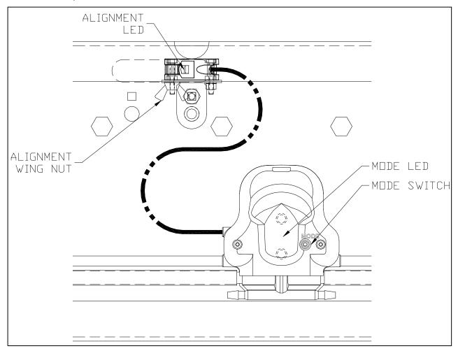
Figure 2: Logic Assembly Mode & Alignment
