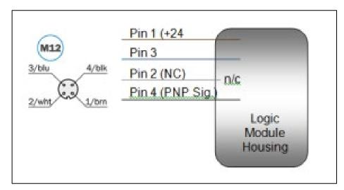
Figure 24: M12 Sensor Connection Pin-out
