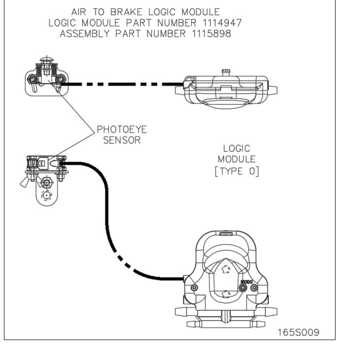
Air to brake logic module - Straight Beds
