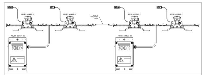
Figure 10: One CRUZcontrol Section with Two Power Supplies
