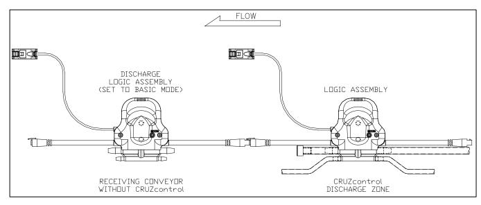
The following hardware listing is for two Discharge Logic Assembly kits consisting of the Discharge Logic Assembly, a reflector, and mounting brackets. The mounting brackets provide for the mounting of the Discharge Logic Assembly and reflector either  $\frac{1}{2}$ " or 3" above a standard CRUZ side channel. Since every application is different, there will usually be a need to drill mounting holes for the brackets.
