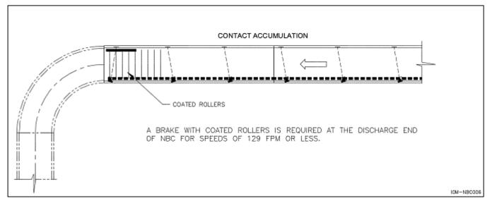
For speeds up to 129 FPM, a brake with six coated rollers is sufficient. Standard brake kits are available for NBC.
