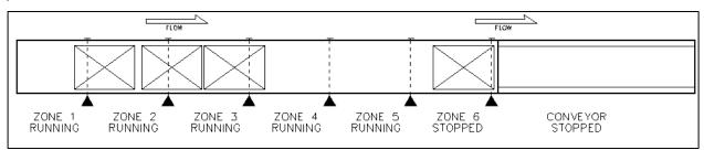
In the above example, the discharge zone, Zone 6, is shown stopped which is the result of the release from the zone being inhibited (receiving conveyor is stopped) and the Zone 6 sensor being blocked.
