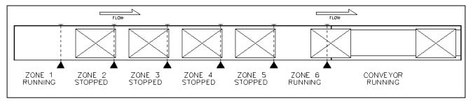
This will create a one-zone length gap between all released products; assuming conveyor speeds (accumulation conveyor and downstream conveyor) are identical.
