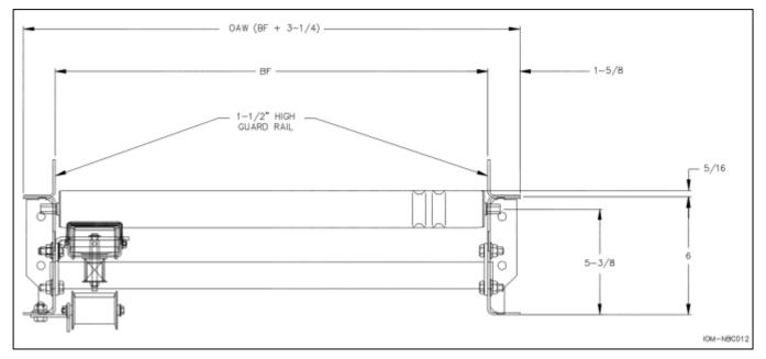
Use 1-1/2" angle for C6 channel guardrail
