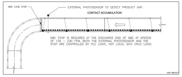
For speeds from 130 FPM to 230 FPM, a stop is recommended at the discharge end of NBC to stop the coasting product and begin accumulation. Standard stop assemblies are available for NBC. Please note that a stop cannot be allowed to come up under a product. An external PLC controlled sensor must be used to detect a gap and then activate a solenoid to raise the stop.
