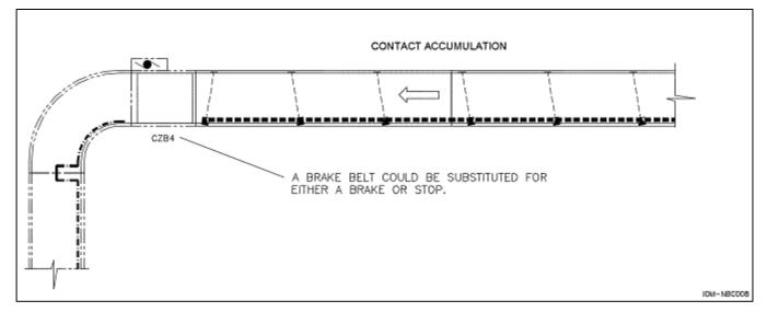
A belt unit downstream can be used in place of either a brake or a stop. If this belt option is selected, use the CRUZ<sup>®</sup> belt 4 series.
