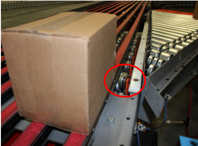
Wrong alignment - missed contact with the first spur side divert wheels.
